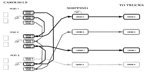
PICK AND PASS WITH CONTINUOUS BATCHING
