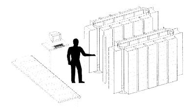
The pod enhances system throughput by allowing the operator to work with several machines simultaneously. All the equipment in the pd is under the control of software, resident on a computer workstation. Even as the operator is handling product at one carousel, the software is positioning another machine for the next item. Product thus moves in a continuous flow.
